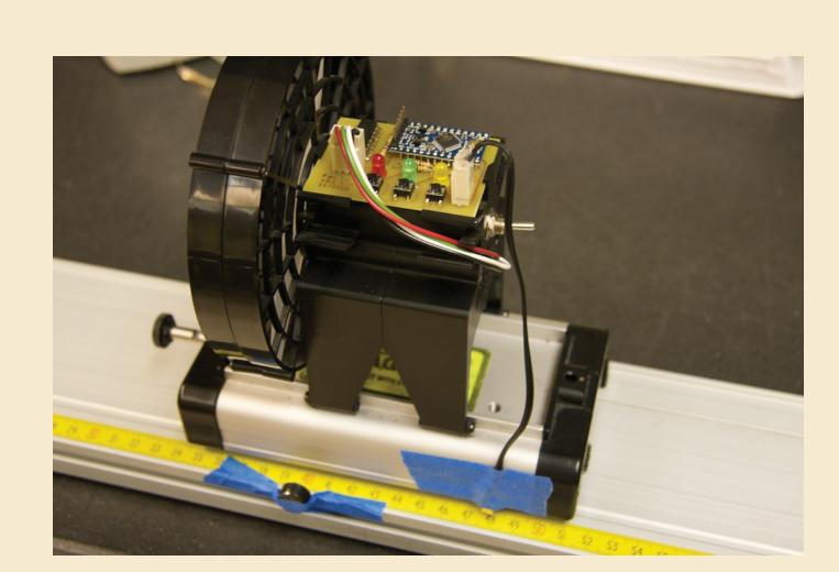
Want to build this for less? If you're comfortable with (or willing to learn) in-system programming, it's possible to build a functionally equivalent circuit using an ATtiny84 and an LM78LOS voltage regulator instead of the Arduino board. This cuts the component cost roughly in half, while still allowing complete control over all aspects of the fan behavior. Contact me for an EagleCAD layout of this circuit if you're interested.
